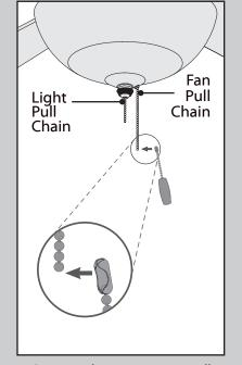
Connect the appropriate pull chain pendant to each of the short chains coming from the finial and finial cap. The fan pull chain controls the speed: from high to off. The light pull chain controls the light fixture: on and off.
