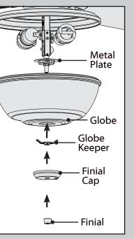
Press the globe and globe keeper flush against the metal plate. Thread the light pull chain through the hole in the center of the finial cap and thread the fan pull chain through the hole in the side of the cap. Finally, thread only the light pull chain through the hole in the finial and screw the finial onto the threaded rod.
