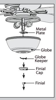
**Changing the bulbs** - unscrew the finial and remove it from the threaded rod. Remove the finial cap and unscrew the globe keeper while supporting the globe with your other hand. Carefully remove the globe. Unscrew bulbs and replace with bulbs of same type and wattage. Reinstall the globe assembly.
