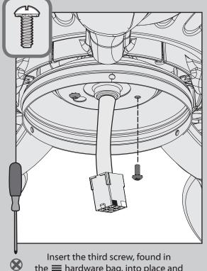
the  $\equiv$  hardware bag, into place and then tighten all three screws.
