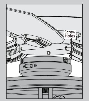
Lift the lower switch housing up until its screw holes are aligned with the screw holes in the upper switch housing.
