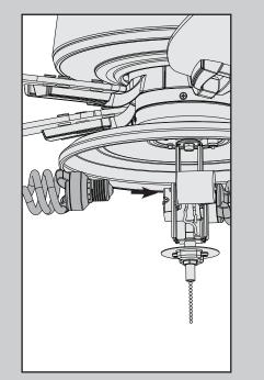
Install a bulb into each of the sockets. When necessary, replace with bulbs of the same type and wattage.
