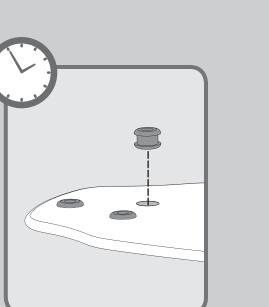
Time Saver Tip: Get a helper to insert grommets, found in the ■ hardware bag, into the blades while you're doing the next couple of steps.
