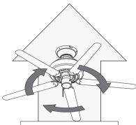
Updraft (clockwise rotation) creates a more indirect airflow. Updraft airflow is great for moving warm air downward.
