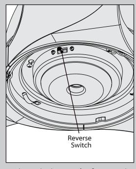
To change the direction of air flow, move the reverse switch to the opposite position. You must remove the globe or no-light cap in order to access the reverse switch.
