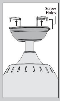
Lift the canopy or Low Profile canopy into place so that the screw holes are aligned.
