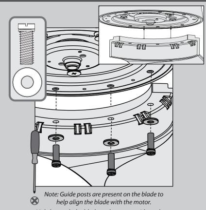
Lightly attach the blade to the motor with washers found in the  $\triangle$  hardware bag and the screws you saved from page 6. Then, securely tighten after all three screws are attached.
