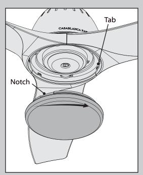
Position the notches in the outer rim of the globe so they line up with the tabs on the inside rim of the upper switch housing. Carefully lift the globe then rotate clockwise until it is held tightly in place by the tabs.
