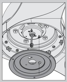
Feed the wire plug through the center hole of the upper switch housing, then wrap keyhole slots around the screws and twist clockwise.
