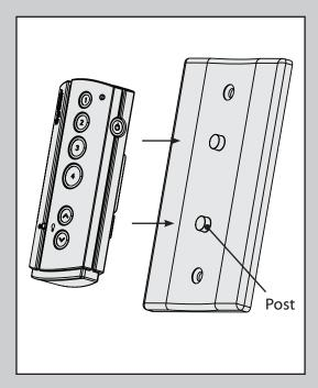
Your Universal Remote comes with a wall plate that has two posts on which to mount your transmitter when not in use.
