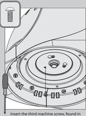
Insert the third machine screw, found in the hardware bag, into place and then tighten all three screws.
