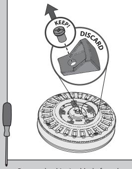
Remove the shipping blocks from the motor. Save the screws. You will need them to install the fan blades.
