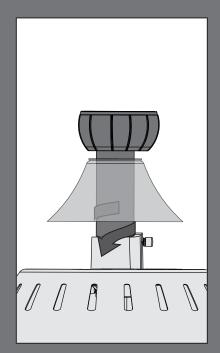
Slide the adapter cover onto the downrod (for standard mount only), then hand tighten the downrod at least 4-5 full turns until it stops.
