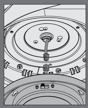
Connect the 9-pin plugs from the upper switch housing and light kit assembly. Make sure to line up the colored markings on the connectors.
