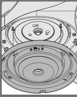
Wrap the keyhole slots around the screws and twist the light kit assembly clockwise.
