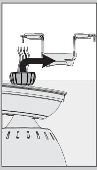
THE CANOPY OR WIRES. Place the downrod ball into the slot in the ceiling bracket.
