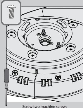
Screw two machine screws
