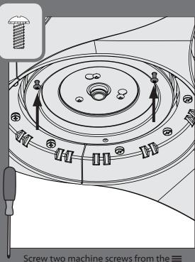
Screw two machine screws from the hardware bag halfway into the upper switch housing. It does not matter which two screw holes you choose.
