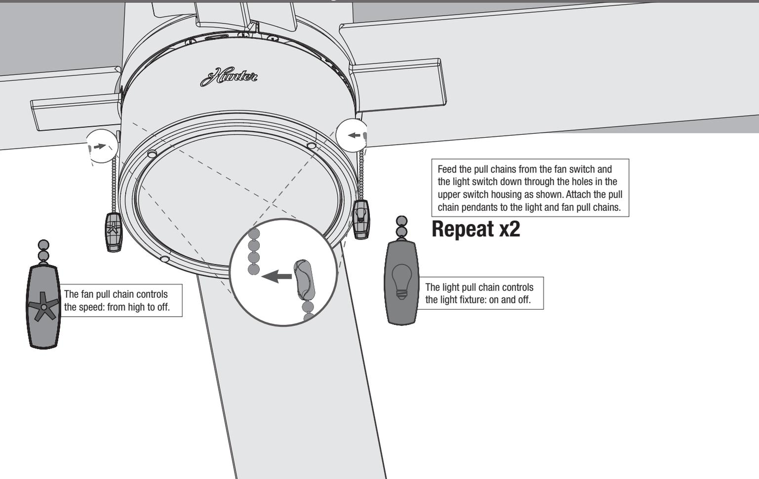
Feed the pull chains from the fan switch and the light switch down through the holes in the upper switch housing as shown. Attach the pull chain pendants to the light and fan pull chains.
