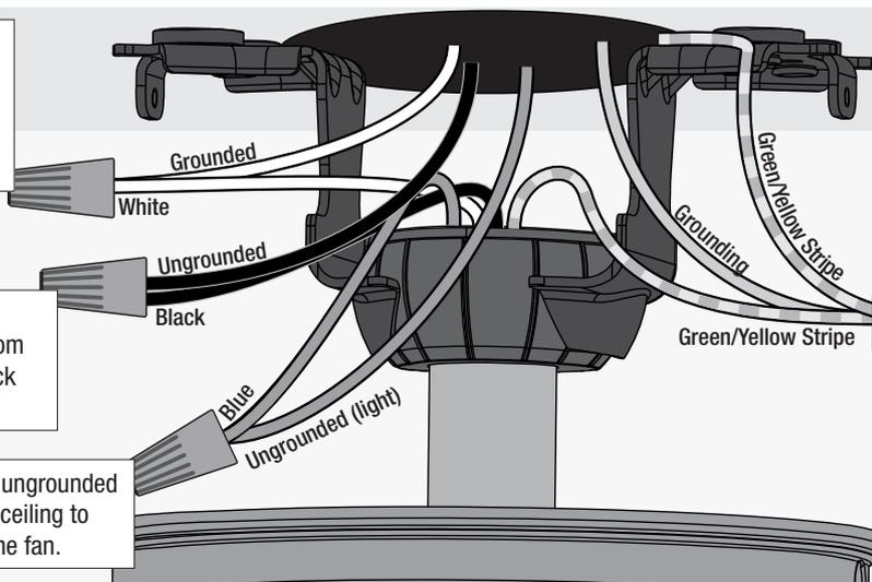
Connect the black (ungrounded) wire from the ceiling to the black wire from the fan.
