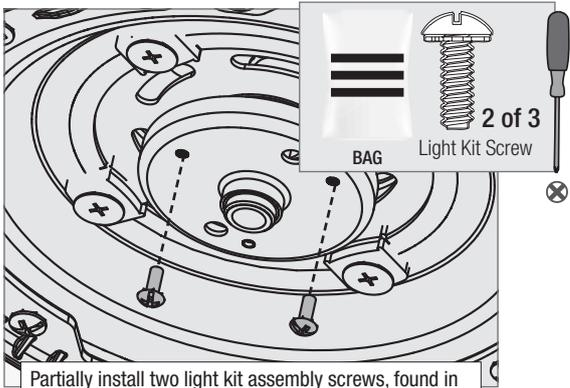
Partially install two light kit assembly screws, found in the
