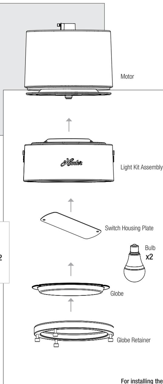
For installing the light fixture
