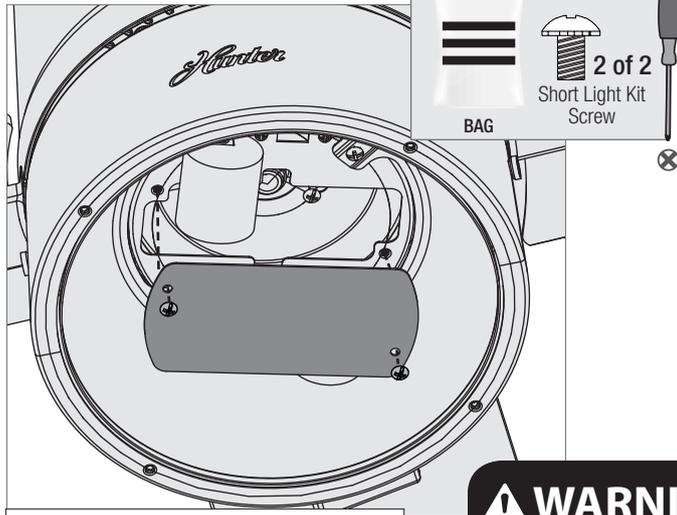
Carefully push all switch housing components into the switch housing, then install the switch housing plate using two short light kit assembly screws, found in the
