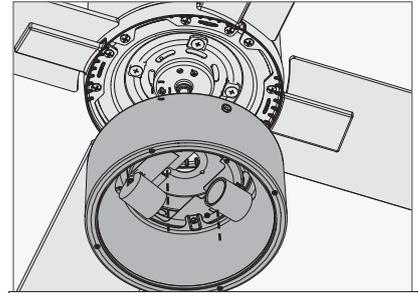
Align the keyhole slots in the top of the light kit assembly with the partially installed assembly screws. Wrap the keyhole slots around the screws and twist counterclockwise.
