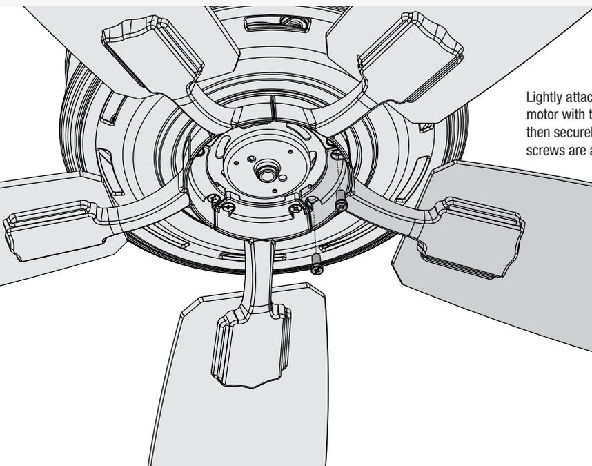
Lightly attach the blade arms to the motor with the blade arm screws, then securely tighten after both screws are attached.
