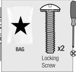
Once the motor is in the ceiling bracket, use the two locking screws found in the ★ hardware bag to secure the motor to the ceiling bracket.
