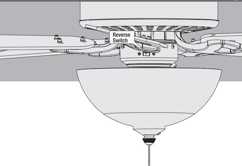
Ceiling fans work in two directions: downdraft (counterclockwise rotation) and updraft (clockwise rotation). To change the direction of air flow, turn the fan off and let it come to a complete stop. Slide the reversing switch to the opposite position. Restart the fan.
