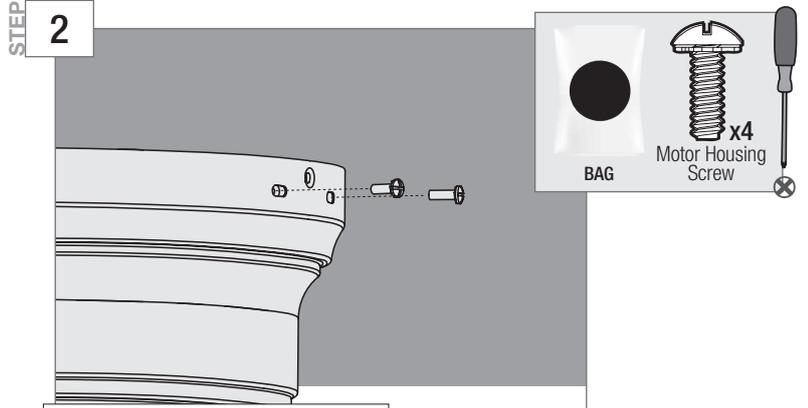
With a Phillips head screwdriver, install the four motor housing screws found in the ● hardware bag. Tighten all four screws securely.
