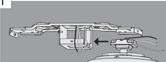
While holding the wires out of the way, lift the motor assembly and place the square hanger into the opening in the ceiling bracket. Be sure the ground wire attached to the hanger faces out of the large opening in the ceiling bracket.
