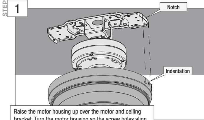
Raise the motor housing up over the motor and ceiling bracket. Turn the motor housing so the screw holes align and the indentation in the housing locks into place with the notch in the ceiling bracket. **The motor housing is not secured until the next step is complete. Do not leave unattended.**
