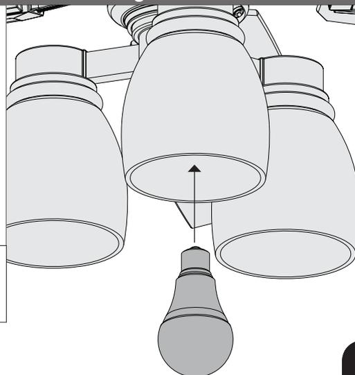
Install a bulb into each of the sockets. When necessary, replace with bulbs of same wattage.
