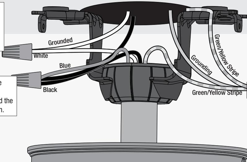
**⚠ WARNING** The ceiling fan must be grounded. If the ground wire for the installation site is not present, immediately **STOP** installation and consult a qualified electrician.
