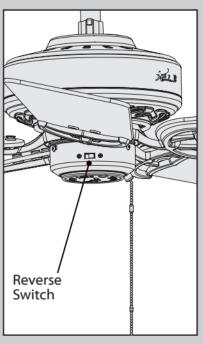
Changing the direction of air flow - move the reverse switch to the opposite position.
