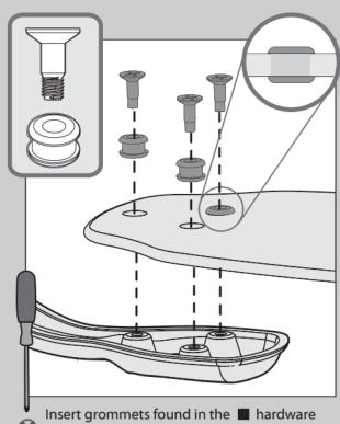
bag into the holes in the blades, then secure each blade to a blade iron with screws found in the **A** hardware bag.
