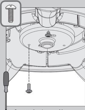
Screw two housing assembly screws the motor housing. It does not matter which two screw holes you choose.
