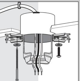
Use wood screws (included) when securing to support structure with approved electrical outlet box. Drill 9/64" pilot holes in support structure to aid in securing ceiling bracket with hardware found in the  $\bigstar$  hardware bag.
