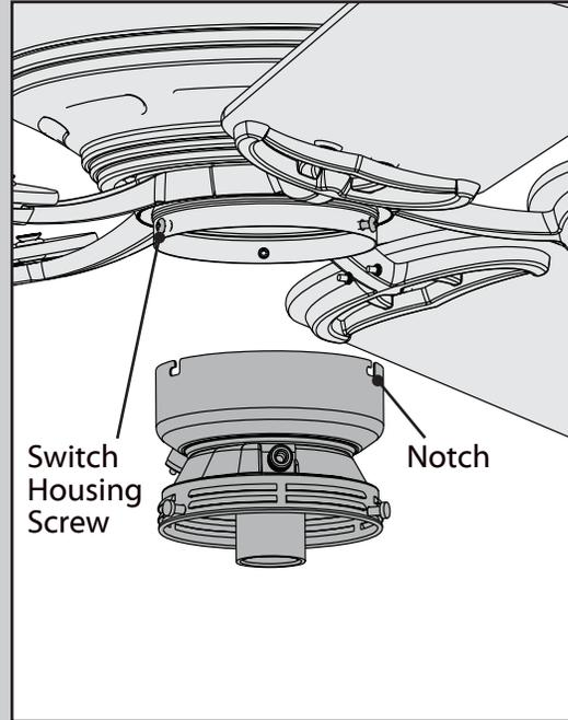
Align the notches in the sides of the lower switch housing with the upper switch housing screws. Lift the lower switch housing. Twist the lower switch housing clockwise to lock into place.
