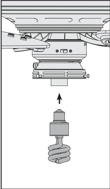
Install a CFL bulb (19-watt maximum).
