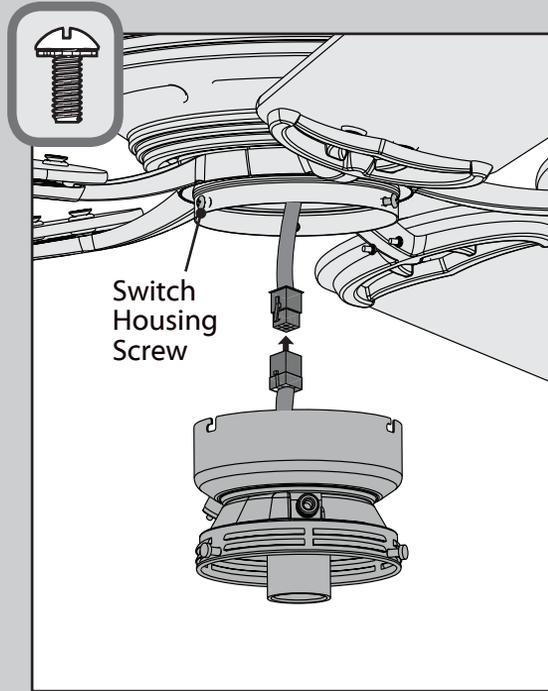
Partially install two of the switch housing screws found in the
