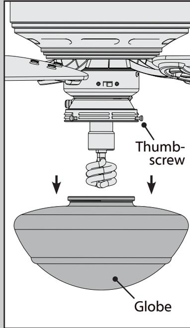
**Changing the bulb** - unscrew the thumbscrews while supporting the globe with your other hand. Carefully remove the globe. Unscrew the bulb and replace with a bulb of same type and wattage. Reinstall the globe assembly.
