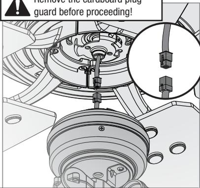
Connect the plugs from the fan and light fixture. Make sure to line up the colored markings on the connectors.
