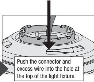
Push the connector and excess wire into the hole at the top of the light fixture.
