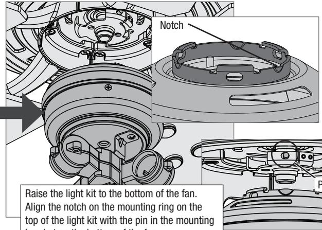
Raise the light kit to the bottom of the fan. Align the notch on the mounting ring on the top of the light kit with the pin in the mounting bracket on the bottom of the fan.
