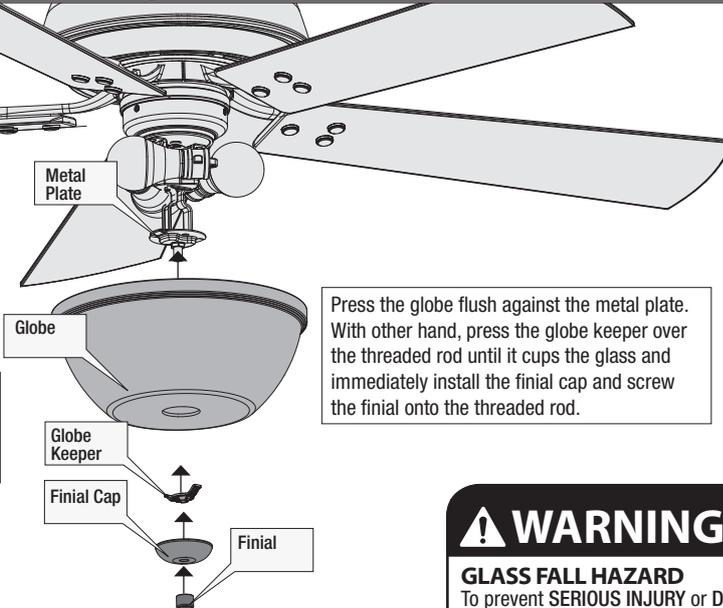
Press the globe flush against the metal plate. With other hand, press the globe keeper over the threaded rod until it cups the glass and immediately install the finial cap and screw the finial onto the threaded rod.
