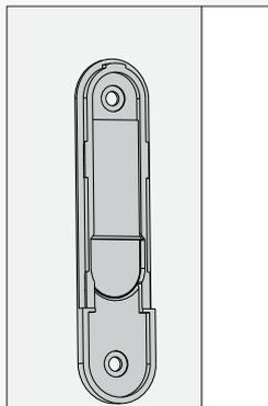
Press the cradle bracket against the wall and hold firmly for 30 seconds.
