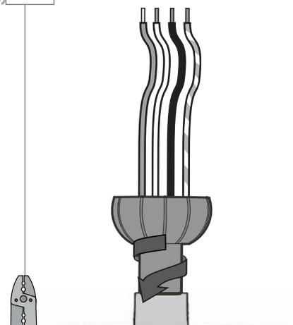
Pass all wires to one side of horizontal bar in downrod assembly. Hand tighten the downrod (at least 4–5 full turns) until it stops. Trim the wires coming from the fan so that 8-inches remain coming from the top of the downrod.
