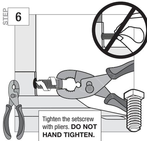
Tighten the setscrew with pliers. **DO NOT HAND TIGHTEN.**
