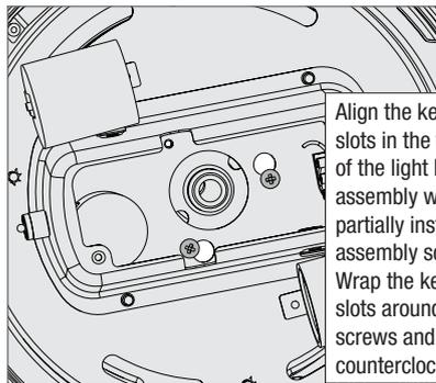
Align the keyhole slots in the top of the light kit assembly with the partially installed assembly screws. Wrap the keyhole slots around the screws and twist counterclockwise.
