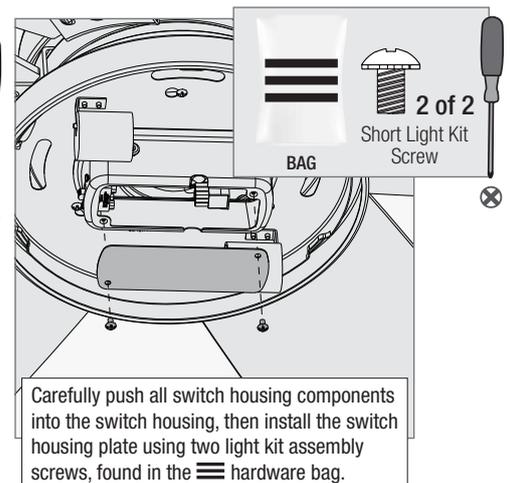
Carefully push all switch housing components into the switch housing, then install the switch housing plate using two light kit assembly screws, found in the hardware bag.
