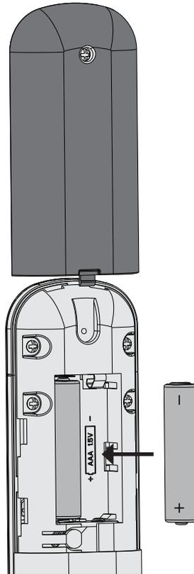
Install two AAA batteries, found in the remote control hardware bag, into the transmitter. Clean the battery contacts prior to installing the batteries. Please contact your local battery recycling center for proper battery disposal information.
