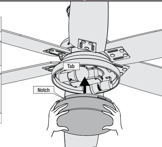
Lift the globe and align the notches in the globe with the tabs in the light kit.
