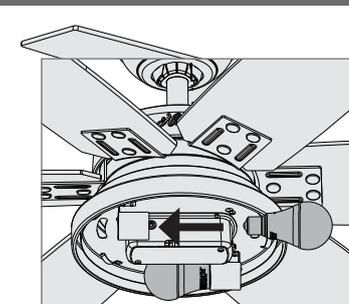
Install the included LED bulbs into the sockets. When necessary, replace with bulbs of same wattage.
