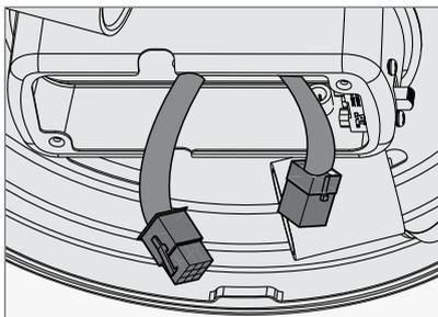
Feed the 9-pin plug connector coming from the bottom of the motor housing through the center hole in the light kit assembly. Connect it to the plug connector found in the switch housing area of the light kit assembly. Make sure to line up the colored markings on the connectors.
