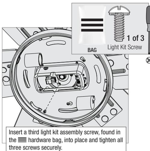
Insert a third light kit assembly screw, found in the hardware bag, into place and tighten all three screws securely.
