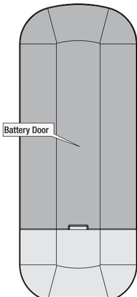
To access the battery compartment, remove the battery door to the transmitter assembly.
