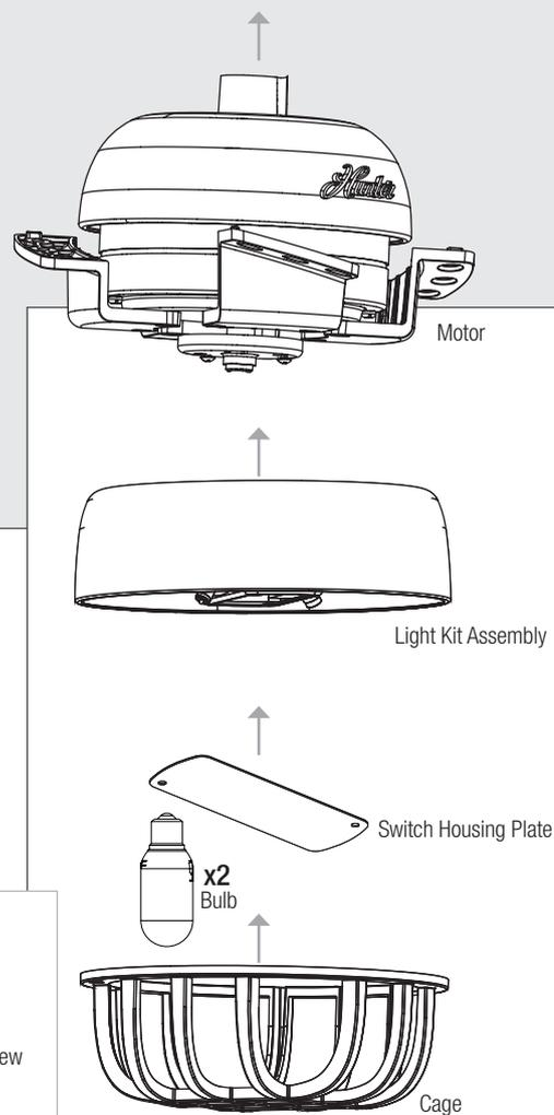
For installing the light fixture
