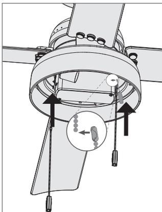
Remove and discard the plastic connectors from the ends of the short pull chain. Attach the pull chain pendants to the light and fan pull chains.
