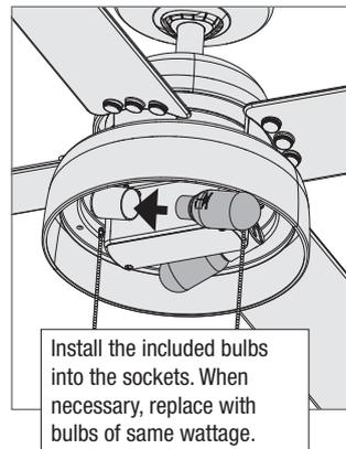
Install the included bulbs into the sockets. When necessary, replace with bulbs of same wattage.
