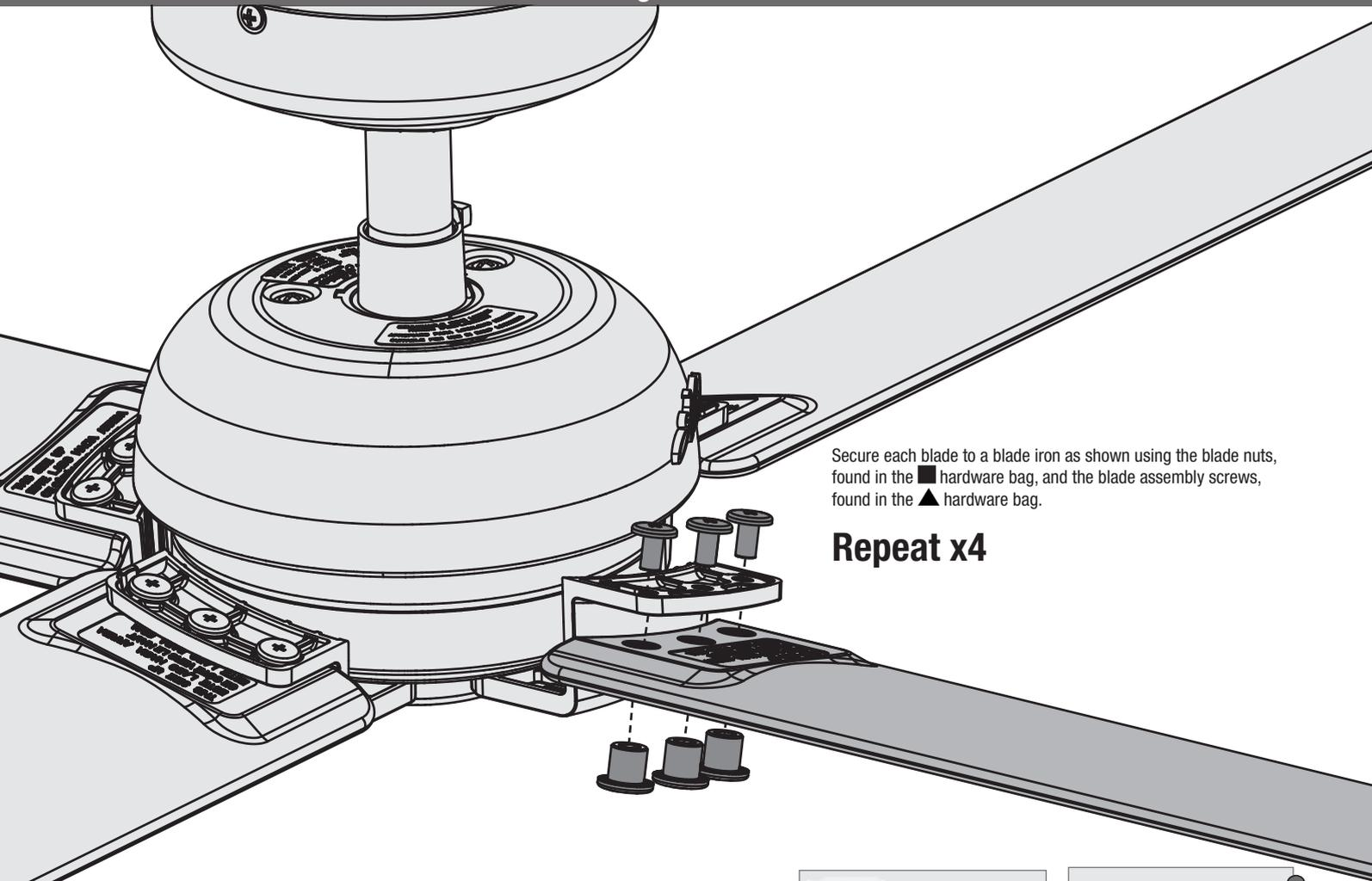
Secure each blade to a blade iron as shown using the blade nuts, found in the ■ hardware bag, and the blade assembly screws, found in the ▲ hardware bag.
