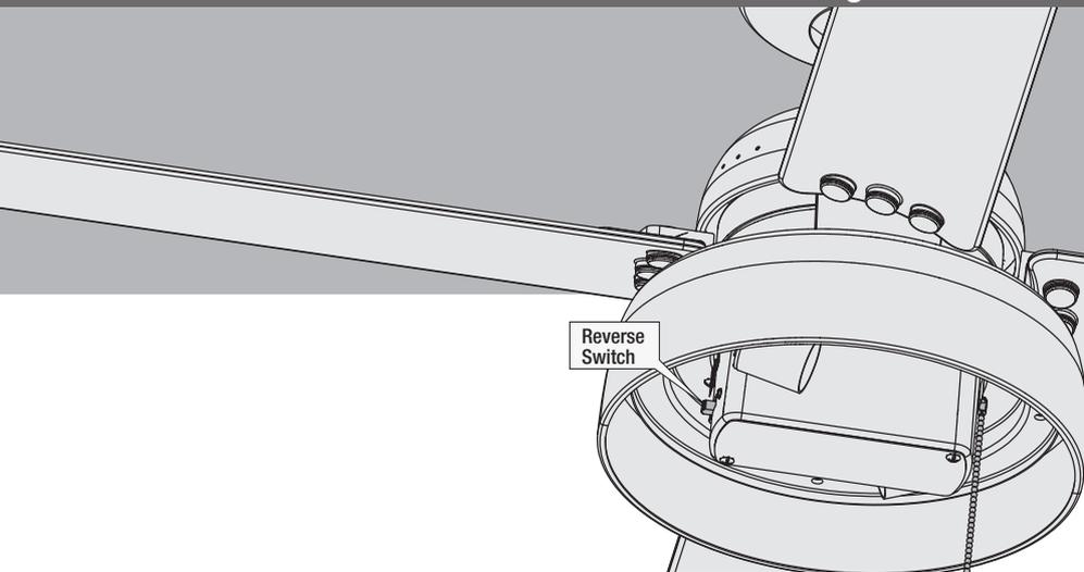
Ceiling fans work in two directions: downdraft and updraft. To change the direction of air flow, turn the fan off and let it come to a complete stop. The reversing switch is located inside the light fixture. It can only be accessed when the cage is removed. Slide the reversing switch to the opposite position. Restart the fan.
