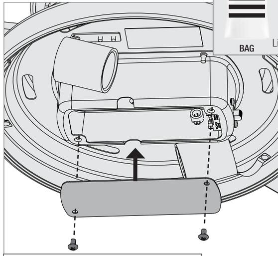
Carefully push all switch housing components into the switch housing, then install the switch housing plate using two light kit screws, found in the hardware bag.
