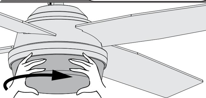
Attach the globe by lifting and turning clockwise one third of a full turn of the glass until it stops.
