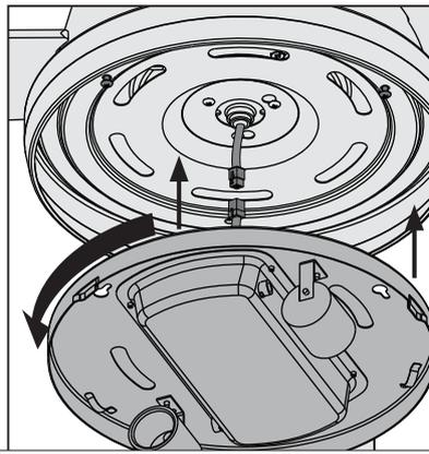
Connect the plugs from the upper and lower switch housings. Make sure to line up the colored markings on the connectors. Wrap light kit keyhole slots around the screws and twist counterclockwise.
