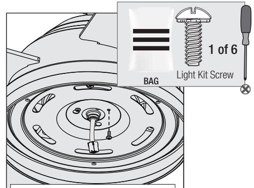
Insert the third screw, found in the hardware bag, into place and then tighten all three screws.
