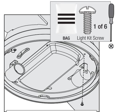
Insert the third screw, found in the bag of materials, into place and tighten the three screws.
