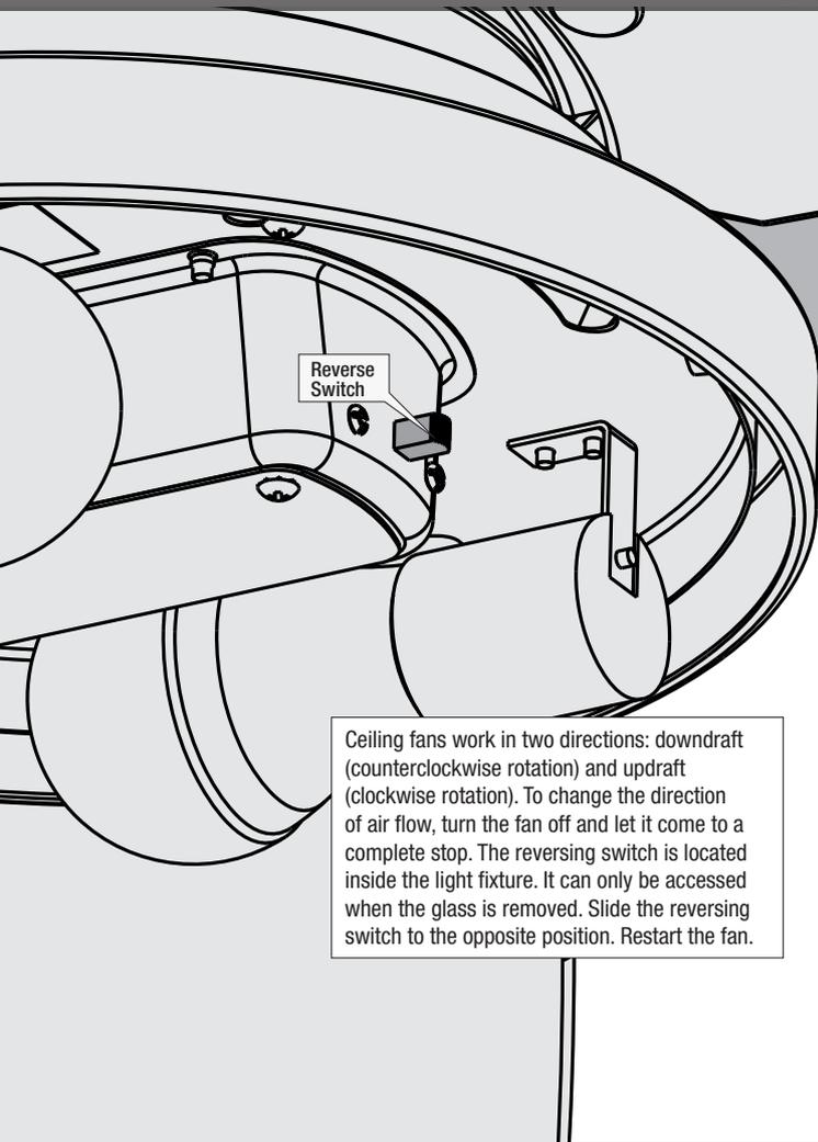
Ceiling fans work in two directions: downdraft (counterclockwise rotation) and updraft (clockwise rotation). To change the direction of air flow, turn the fan off and let it come to a complete stop. The reversing switch is located inside the light fixture. It can only be accessed when the glass is removed. Slide the reversing switch to the opposite position. Restart the fan.
