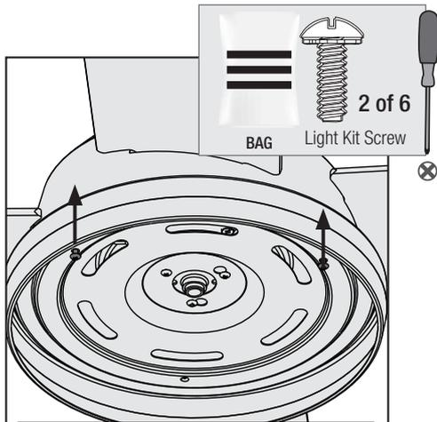
Screw two housing assembly screws from the hardware bag halfway into the upper switch housing. It does not matter which two screw holes you choose.
