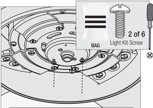
Screw two housing assembly screws from the hardware bag halfway into the motor housing. It does not matter which two screw holes you choose.
